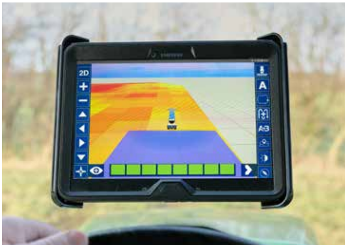
NAVI App for GPS spreading via Android tablet (requires CALIBRATOR ZURF).
