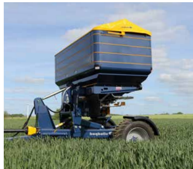
The spreader can be dismantled and used for late top dressing in high crops.
