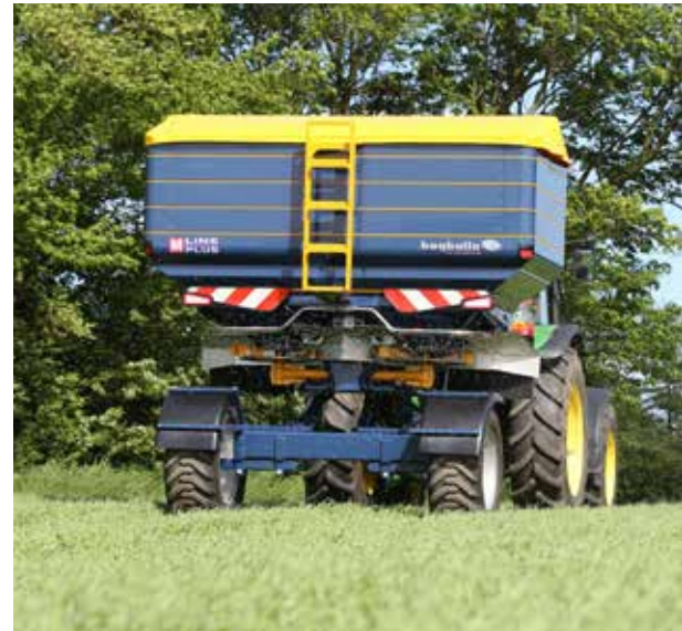
M45-Trail for spreaders up to 4500 Kg.
