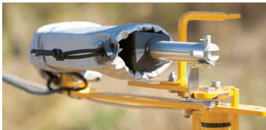
Electric remote control of border spreading for CALIBRATOR ZURF/ICON
