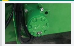
As the floor conveyor works independently from the rotor, this ensures that fodder can be reversed away from the rotor without disengaging the rotor.
