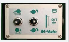
An external loading control comes fitted as standard which will allow for the conveyor floor and the tailgate to be operated when removing the netting or wrap whilst loading a bale. The tailgate and conveyor alignment on the machine body take the largest size square bales without the need for extensions to the tailgate.
