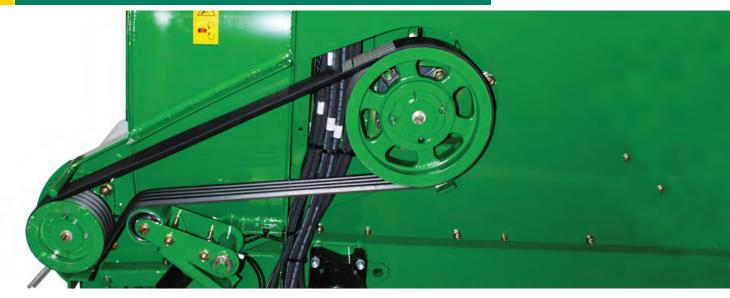
The High Torque Belt Drive, which drives the feed rotor, can be hydraulically engaged or disengaged. This system ensures that the flywheel (straw blowing turbine) can be worked independently of the rotor.
