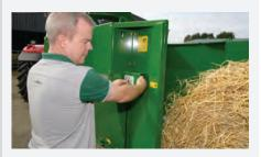
To prevent accidental operation of the controls, a safety button on the side of the External Loading Control must be pressed while operating loading functions at the rear of the machine.
