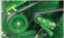
The McHale C4 Silage Feeder & Straw Blower range of machines are designed to allow the rotor work independently from the flywheel. This allows the flywheel to be at full RPM before any fodder material is fed into the rotor.
