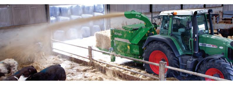
The McHale C4 Silage Feeder & Straw Blower Range is fitted with a three-stage chute. This three-stage design minimises resistance and allows for maximum blow distances to be achieved, especially when blowing straw in confined spaces.
