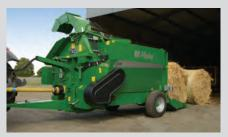
The tailgate on the machine can be used to load a bale without the need for a second tractor. The cupped tailgate design ensures a bale is held in the dip in the tailgate, while the twine or net is being removed. The ram mounting points on the tailgate ensure that maximum lifting power can be achieved so that the heaviest of bales can be handled.
