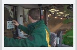
The chute is joystick controlled, allowing the operator to adjust the chute height and the shoot direction easily from the control console in the tractor cab. The chute can be rotated 300°, which allows material to be spread on the left, right and behind the machine. The chute may also be lowered to blow material on to the feeding slide for better control when distributing feed along a barrier.
