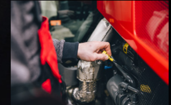
Front axle and slim waist bonnet design make oil dipstick and filter access easy.
